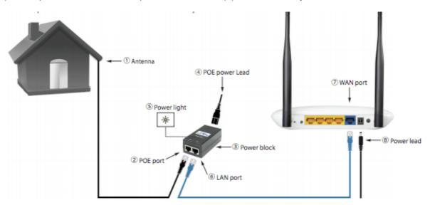
Sometimes simply turning the router odd and on will resolve most issues. To do this disconnect the power lead (8) from the rear of the router, you will see the lights displayed on the front of the router turn off. Leave it for around 5-10 seconds before plugging the power lead (8) back in and turning the router back on. Wait an additional 60 seconds and try the connection on your device again.
